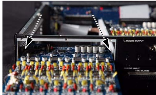
Inserting the card into the guide rails for the empty bay
