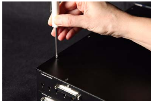
Removing the top cover screws
