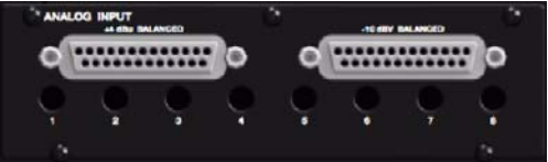
+4 dBu and –10 dBV DB-25 Analog Input ports
